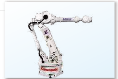
Welding robot produced by Kawasaki Heavy Industries Ltd.
